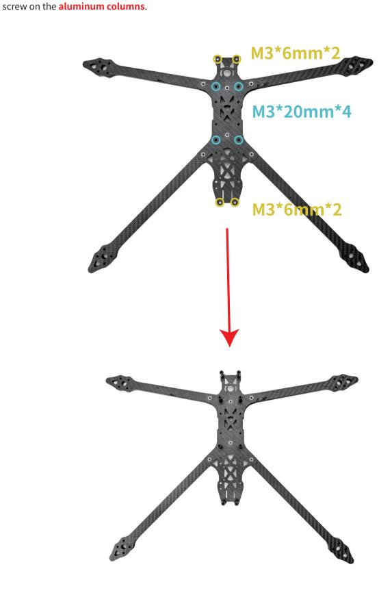
④Attach the two lens prints and one tail print to the aluminum post as shown.screw on the aluminum columns.
