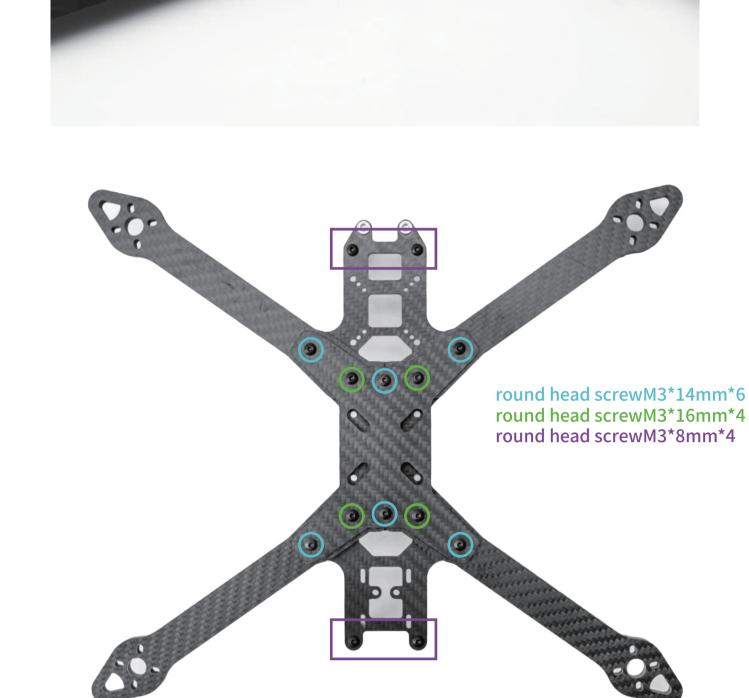
Screw on the aluminum posts for the eight screws indicated in the diagram.
