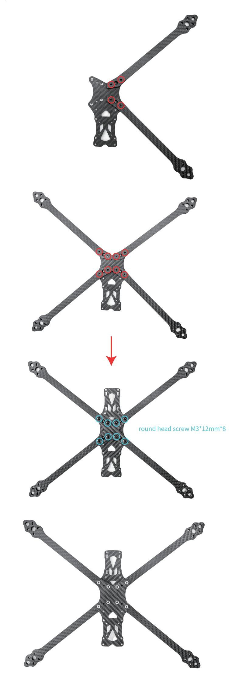
Screw in the eight holes marked in the diagram and screw in the aluminum posts on the backside
