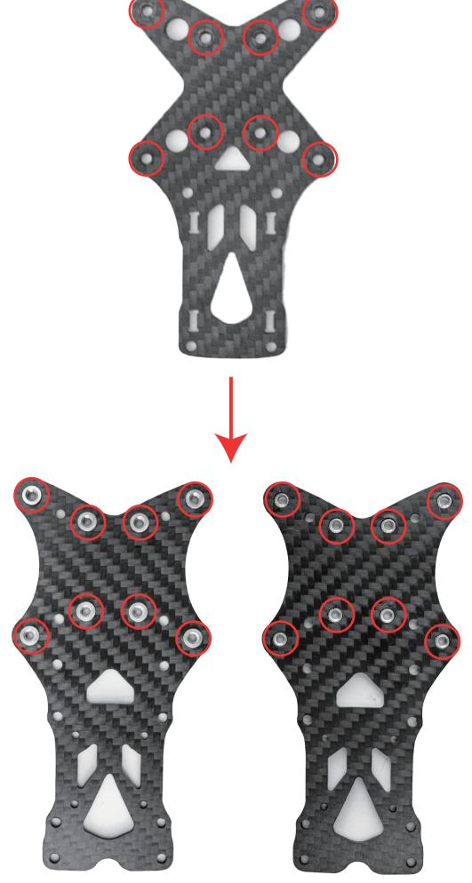
Sandwich the arm between the base plate and the center plate in the order shown in the diagram and drive screws in the eight holes marked on the base plate
