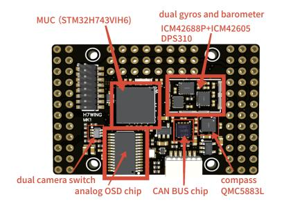
FC board(bottom layer) layout diagram
