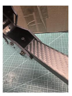
Fix the side of the arm with two screws (④.2) and two locknuts (④.3) as shown in the figure.
