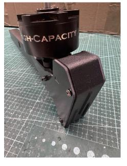
Secure the print between the left and right plates with the screws (③.3).
