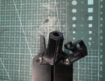
Separately mount the two prints on the upper plate of the tail end as shown in the figure and drive one screw each (2.6, 5.1)
