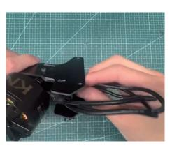
Tuck the motor wires into the arm and lead out the other side
