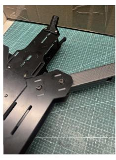
Individual arm to fuselage connection complete!
