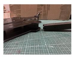
Insert the arm into the fuselage and align the holes
