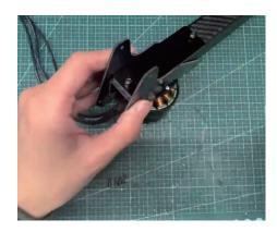
Fix the left and right plates with screws (3.1, 3.5).
