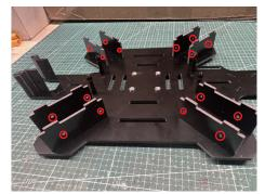
Install arm reinforcement side plate \*8 as shown (pay attention to the orientation)
