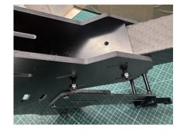
Secure the arm with two screws (④.1), two locknuts (④.3) and two washers (④.4).
