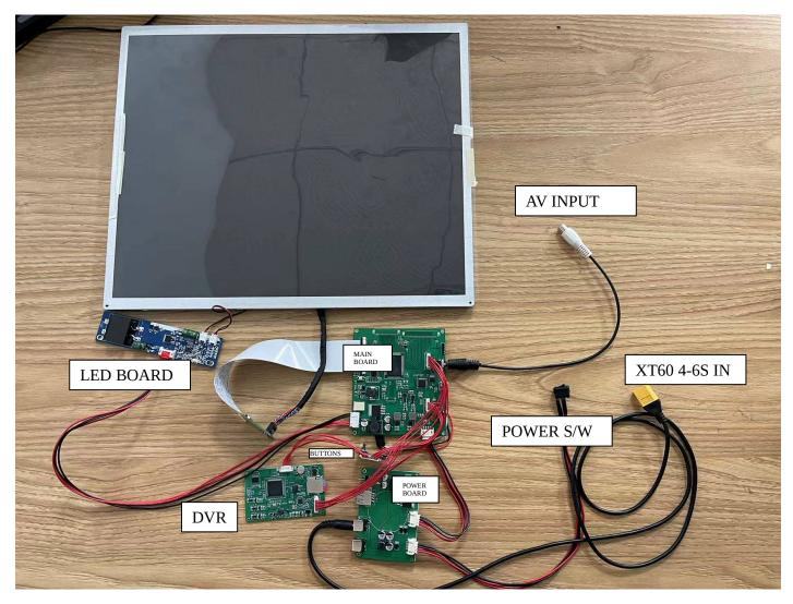
**Modify**: Monitor cable connect directly to main board(NOTE the red wires side to the board center):
